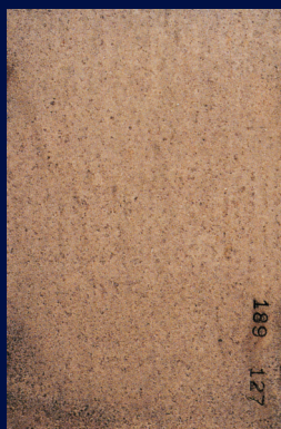
Galvalume test panel shows only moderate edge discoloration after 23 years in same rural environment.
