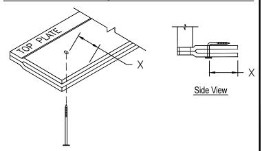
Tool bending depth can be modified by simply drilling a  $\frac{3}{16}$ " hole through each end of the Hemming Tool plates at desired depth dimension "X", then install a Ring Shank Roofing Nail in each end of the tool, up through plates, and bend over Nails. Nail heads should be on bottom plate.
