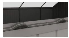
**Step 2:** The inside Closure fits the underside of the panel.
